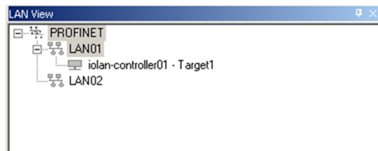
Figure 50: Adding a New LAN to the Configuration
