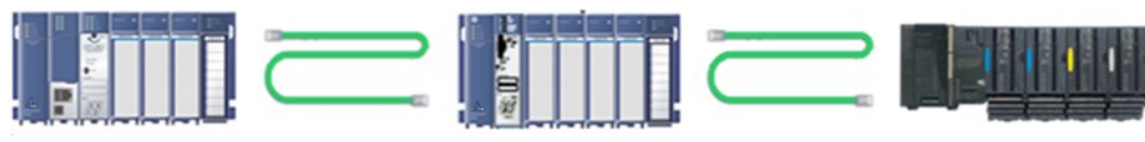
Figure 23: Interconnect using Copper Cables / RJ45 Connectors
